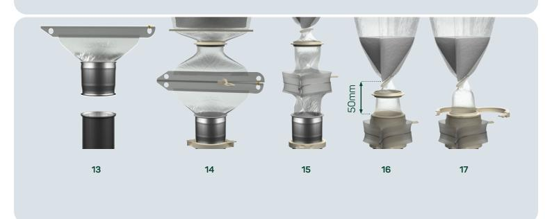
Important: Please always pull, not push, the zips over the transfer tube. Otherwise, the zips could potentially become deformed which could lead to uncontrolled opening of the system.
