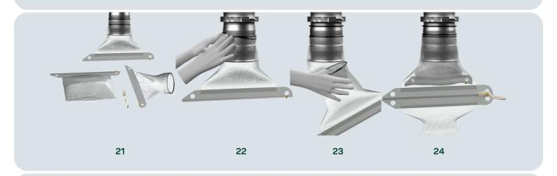
Important: Please always pull, not push, the opened zips over the transfer tube. Otherwise, the zips could potentially become deformed which could lead to an uncontrolled opening.
